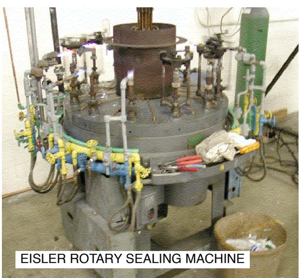
EISLER ROTARY SEALING MACHINE
