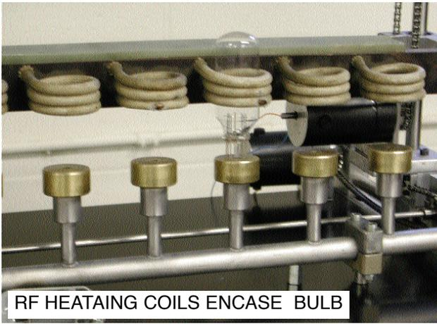
RF HEATAING COILS ENCASE BULB
